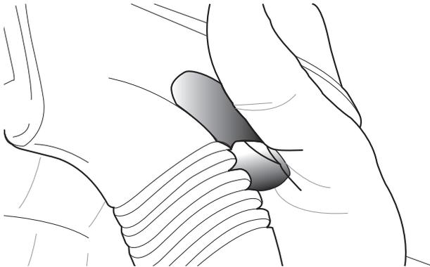
**Too Tight:** Shaded area of handle (above) should seat comfortably into shaded area of hand between thumb and index finger.
