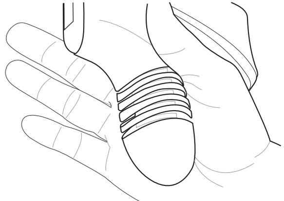
**Proper Fit:** Handle rests on top of hand. Seats into area between thumb and index finger without pinching, and rests in palm without wobbling when shaken lightly.
