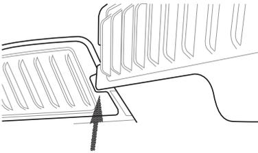
**REMOVE CARTRIDGE:** Use the pointed tip from loose cartridge to pop out existing cartridge. Little force is needed.
