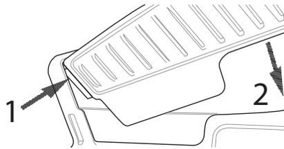
**INSERT CARTRIDGE:** Put tongue on front of cartridge under lip at front of handle (1), then rotate cartridge down (2) and inward (3) to lock in place.
