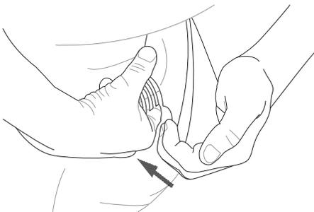
To widen handle, lock front end against your hip and grab with a clawed grip (above) and pull bottom of handle away from top as shown. This will take force. There is a high-strength aluminum rod running top to bottom that will bend. Test fit and repeat until proper fit is made.
