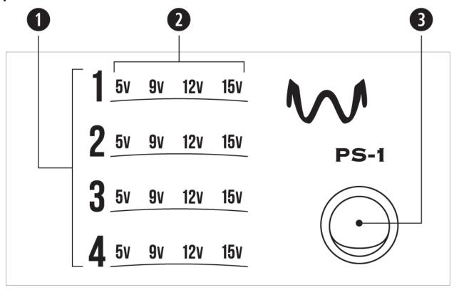
The front panel display tells the user which power zones are being used (1, 2, 3, 4) and which voltage is set per power module (5v, 9v, 12v or 15v). If a power module is added, removed and/or a voltage is changed, the display will update automatically.
