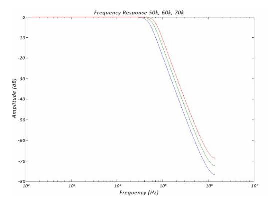
The Roll-off slope setting configures the PCM filter as pictured below in the 20-20kHz frequency sweep.
