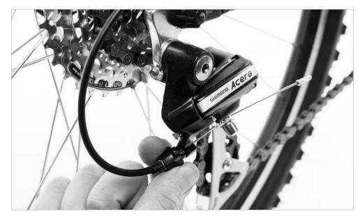
To adjust the dérailleur cable tension, shift the chain onto the smallest sprocket and try to shift on to the second sprocket by changing the gear on the handlebar.
