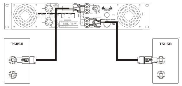
**Attention:** The impedance of connected speaker must match the impedance of amplifier output.
