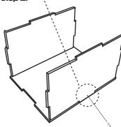
Take one of the panels with a handle and attach it to the shorter end, between the two previously added panels.
