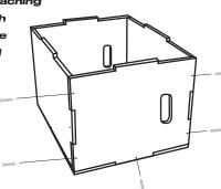
Slide the middle support pieces together and screw in place to keep secured.
