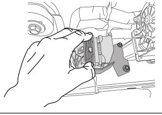
Attach wire harness to controller (make sure connector locking tabs fully engage). Mount controller with the two 11" tie wraps(13) to factory conduit, just rearward of battery.
