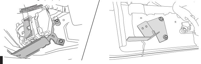
Locate mounting points. First and last set of studs on the inner sill. Motor linkage mounts towards the front of the truck and Idler towards the rear. Driver side shown below.
