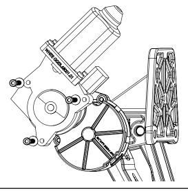
Mount drive and Idler linkage assemblies using supplied conical washer nuts (11) use a 13mm socket or wrench to tighten. Repeat for passenger side. Make sure linkages sit square, fully resting on studs before tightening. Torque to 16ft-lbs (22Nm).
