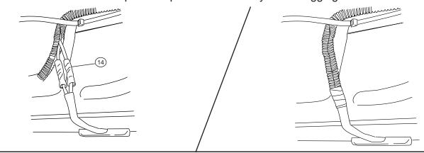
Reinstall Fuse into Powerstep harness. Check that all doors activate the Power Step and the LED Lights work when doors open and close. Reinstall any remaining trim panels. **NOTE:** Verify front linkage clearance at Frame mounted Vibration Dampener. If linkage contacts Dampener in stowed position loosen bolt at pivot point and rotate up to provide at least 1/2" clearance.
