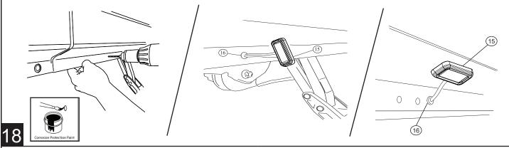
Using supplied butt connectors (14) connect the lamp wires. Red to Red, Black to Black. Once Crimped use heat gun to shrink tube. Close and wrap conduit with electrical tape. Secure all loose wires with cable ties. Pull lamp wires upward to avoid any wire snagging.
