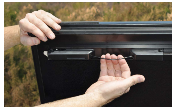
ACCESS RELEASE CABLES ON EITHER SIDE
