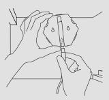
2. Connect the power supply to the rear of a single hexagon.
