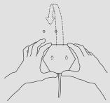
3. Anchor the first hexagon to the wall by using the nail holes on the back.
