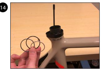
If there is play in the insert when fully tightened down, repeat steps 7-13 using one of the thicker washers supplied with the insert to achieve the proper preload on the insert.
