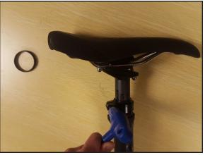
Using an M4 allen wrench, loosen the seat post clamp bolt.
