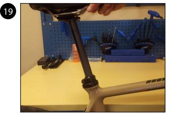
Slide the seat post into the ISO FLEX insert.
