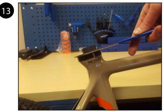
Tighten the lock ring into place using one of the recommended tools. THE LOCK RING SHOULD ONLY BE TIGHTENED UNTIL IT BOTTOMS OUT ON THE SEAT TUBE COLLAR. DO NOT OVER TIGHTEN.
