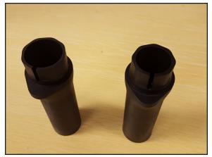
There are two ISO FLEX inserts that can be used on the Vault. One is for a 27.2mm rigid seat post and the other is for a 30.9mm dropper post. Each insert has a size-specific seat post clamp.
