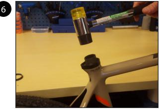
Lightly tap the ISO FLEX insert into the seat tube using a rubber mallet.
