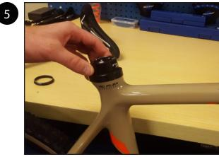
Place the seat post clamp back on the ISO FLEX insert with the lock ring now removed.
