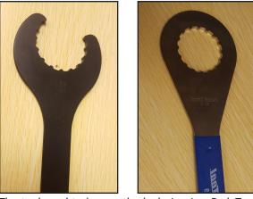
The tool used to loosen the lock ring is a Park Tool BBT-9 or a Shimano Tool TL-FC32.
