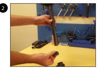
Remove the seat post and seat post clamp.
