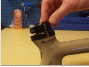
Place the seat post clamp onto the ISO FLEX insert.
