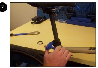
Using an M4 allen wrench, tighten the seat post clamp bolt to 5 [Nm].
