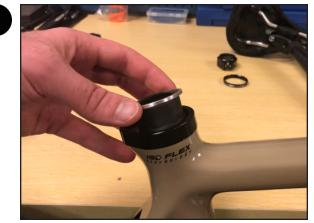
Slide washer over the insert. (If yours does not have a washer then no washer is required).
