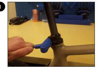
Using an M4 allen wrench, loosen the seat post clamp bolt.
