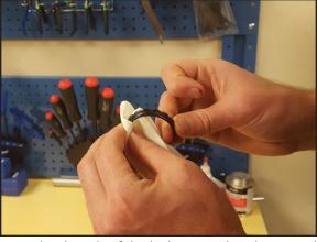
Wipe the threads of the lock ring with a shop towel to remove any dirt or grit.
