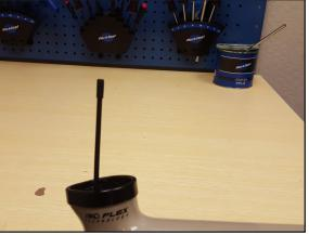
When installing the 30.9mm insert for a dropper post, route the housing through the frame at this point. For the remaining steps, the housing should be routed through the insert during installation.
