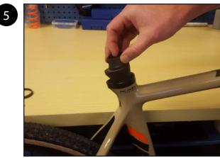
Drop the ISO FLEX insert into the seat tube.
