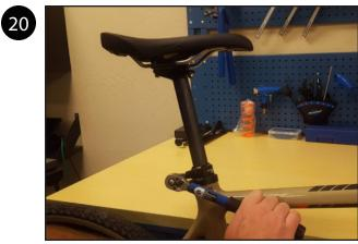
Set the seat post to your desired saddle height and tighten the seat post clamp bolt to 5 [Nm] using an M4 allen wrench.
