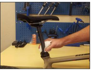
Remove any excess grease from the seat post.
