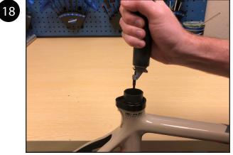
If you are installing a dropper post, connect the dropper post cable at this point.
