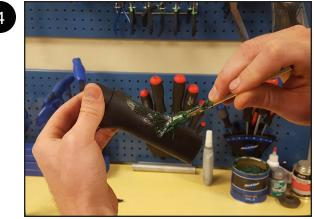
Apply a light layer of grease to the outside of the ISO FLEX insert.
