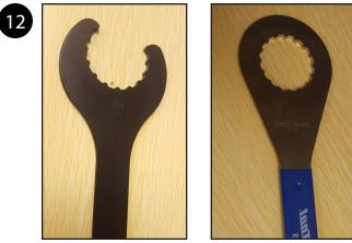
The tool used to tighten the lock ring is a Park Tool BBT-9 or a Shimano Tool TL-FC32.
