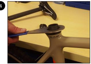
Using one of the recommended tools, loosen and remove the lock ring.
