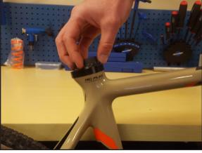
Screw the lock ring onto the seat tube collar by hand. The lock ring should freely thread onto the collar. If there is resistance, unscrew the lock ring and be sure the lock ring isn't cross-threading and try again.
