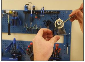
Apply grease to the threads of the lock ring.
