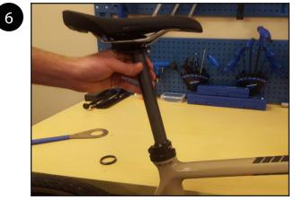
Slide the seat post into the ISO FLEX insert. The saddle height is not critical.
