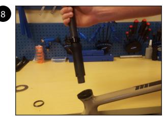
Pull up on the saddle to remove the ISO FLEX insert from the seat tube. A small amount of wiggling to get the insert to release may be required.
