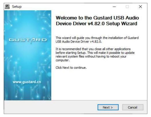
5. When the installer checks the device, if there is a red text prompt: Setup requires that the device is..., please restart the GUSTARD DAC-X16 or re-plug the USB cable.
