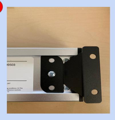
Step 2. Then, pivot the mounting bracket into place so that the bracket locks into the channel and slide it up against the two screws on either end of the bump bar. Tighten the screws installed in step one so that the bracket locks into place.
