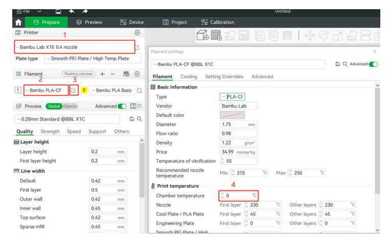
The chamber temperature can be set within the range of 0 °C to 60 °C (the chamber temperature heating control module only operates within the range of 40 °C to 60 °C).
