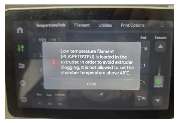
(2) When setting the chamber temperature below 40 degrees Celsius (including 0 °C and other values below 40 °C), it represents disabling the chamber temperature heating control. In such cases, the system will automatically set the chamber temperature target to 0 °C.
