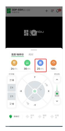
The logic for setting the temperature is the same across all three approaches mentioned. Taking the example of setting the temperature through the printer's screen UI, here is an explanation of how to actively set the chamber temperature. Here are some important points to note regarding chamber temperature settings:
