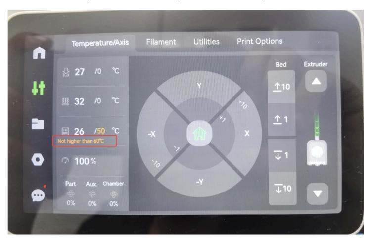
(4) If the current chamber temperature or target chamber temperature exceeds 45 degrees Celsius, it is not allowed to load low-temperature filament (such as PLA, PETG, TPU) to prevent clogging.
