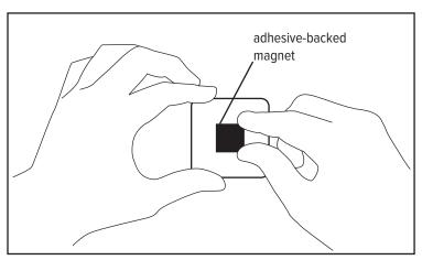
**Step 3:** To complete the magnet, peel the film off the two-sided tape from the magnet back (included) and attach to the magnet.
