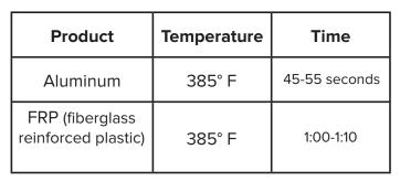
**Step 2:** Press magnets at **385 Degrees F** following the times found in the chart. Increase time if pressing more than one magnet at a time.
