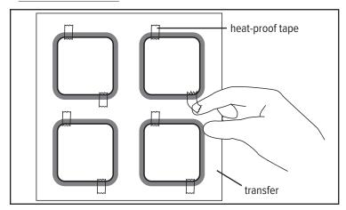
**Step 1:** First, clean the magnet. Next line up and center on transfer and tape magnet to the transfer.
