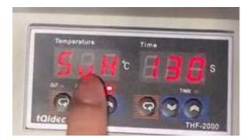
• Then adjust the value of the SVH interface to 248° - 257°F by pressing up or down key.
