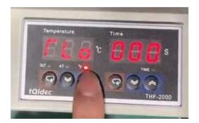
After entering Fahrenheit, you also need to adjust the maximum temperature in the Fahrenheit state.
