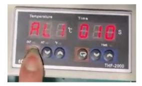
• Press button up button once then finally press the "out" button to save the settings.
