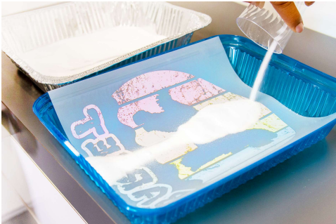
2. Apply shaking powder over the ink using S-POWDER.
