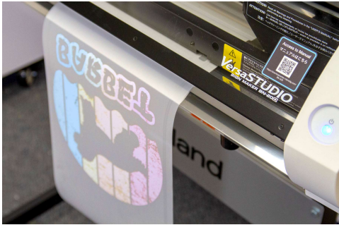
1. Print to film with the BN-20D and S-PG inks, on S-F164 transfer film.
