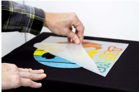
4. Heat press design to your fabric and remove the film backing.
