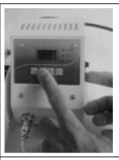
Press the Model Key, at the same time switch on – then C and F can exchange
