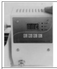
Switch on and it shows C – means the default setting is Degree Celsius.
