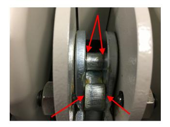
Lubricate these four gaps with small amount of grease. Recommend once a month for normal use.
