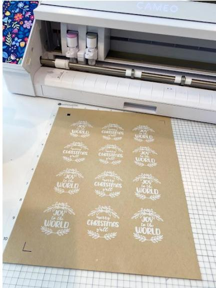
Load the mat and material into the [Silhouette CAMEO](#) by pressing the up arrow on the CAMEO's control panel. Wait for the light to flash, then hold the mat with both hands so it's gently touching the roller bar. It will be fed in after about 3-5 seconds.
