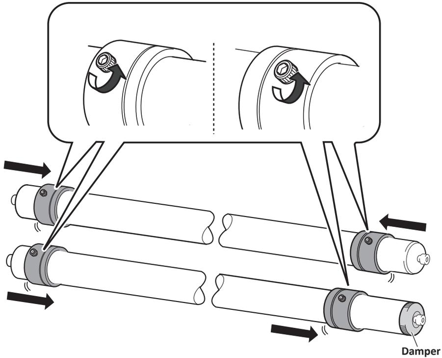
**3 Attach the roll holders to the roll holder supports.**
