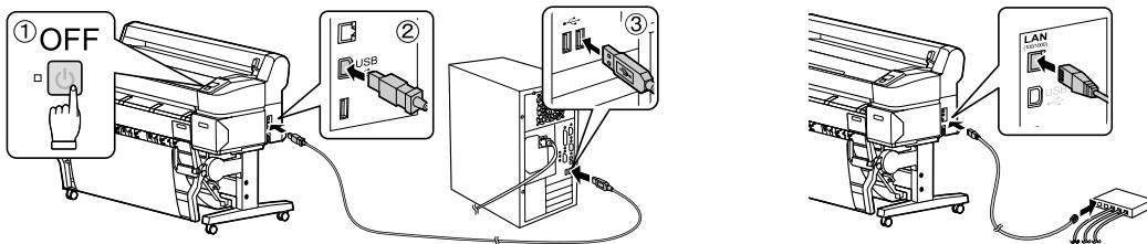
2. Plug the other end of the cable into the appropriate port on your computer or network switch or hub.
