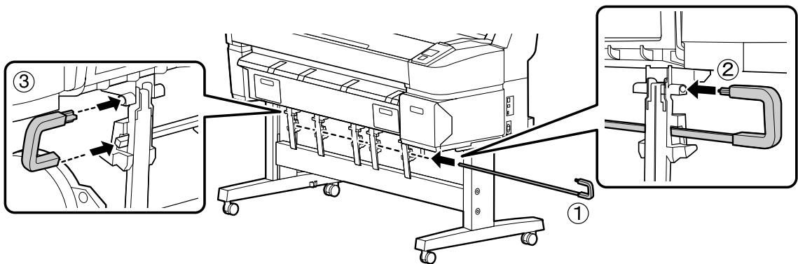
4. Attach the stack guides to the bottom of the printer. Make sure each guide snaps securely into place.
