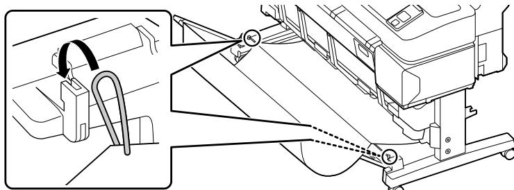
8. Hook the loops on the sides of the basket to the pins on the back of the stand legs to secure the basket to the printer.
