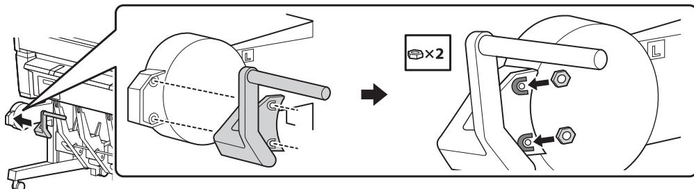
14. Use two bolts to fasten the arm in place.
