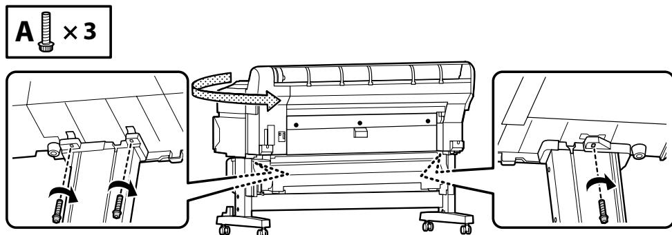
3. Push the second roll unit underneath the printer.
