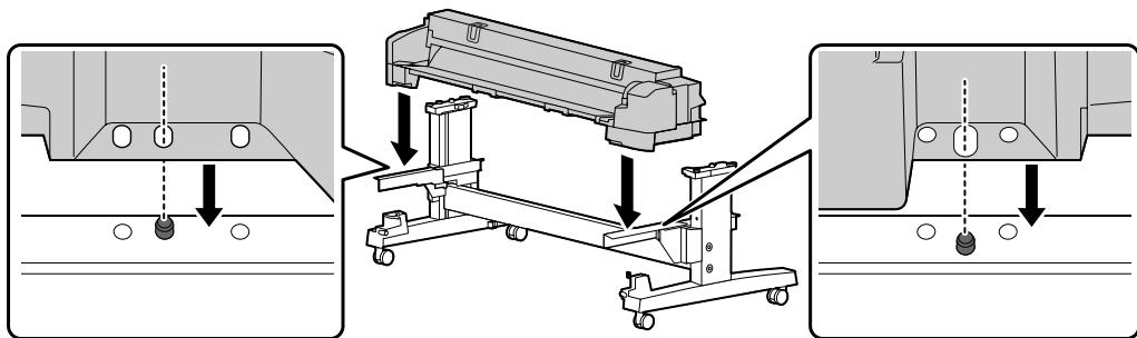
5. Secure the unit to the rails with two bolts on each side.
