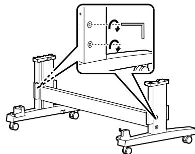
4. Lock the casters to fix the stand in place. (When moving the printer, unlock the casters.)
