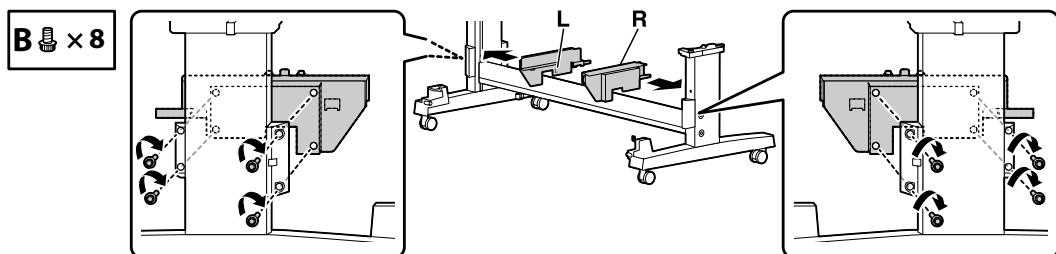
3. Remove the tape from the mounting brackets and extend the left and right rail until you hear a click.
