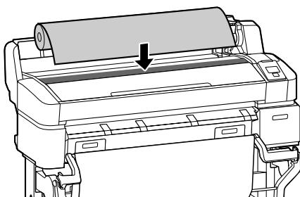
4. If necessary, adjust the roll media adapters to fit the core size of the roll paper.
