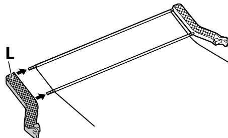
10. Attach the two basket holders, one on each side of the stand. Use four bolts to fasten the holders in place.
