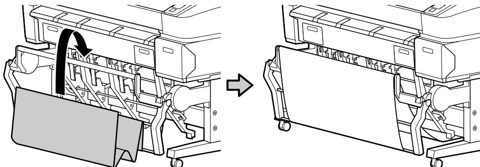
19. On the back side of the printer, pull the paper basket up so that the stack guides fit into the slots as shown. Then, hook the loops around the pins on the back of the stack guides to hold the basket in place.
