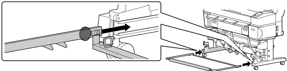
4. Pivot the basket frame and close the rail covers. Replace the bolts.
