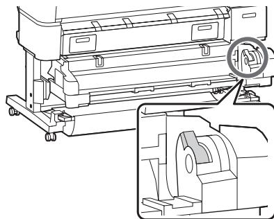
5. Place the roll paper adapters on the adapter guides with the flat side down. Then, slide the paper roll slowly inside.
