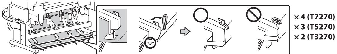
20. Hook the loops on the sides of the basket to the pins on the back of the stand legs to secure the basket to the printer.
