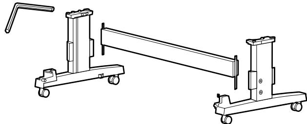
2. Slide the horizontal strut into both of the legs.
