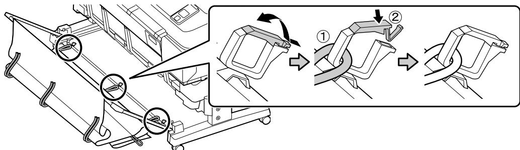
7. Hook the loops on the sides of the bottom of the basket to the pins on the stand.
