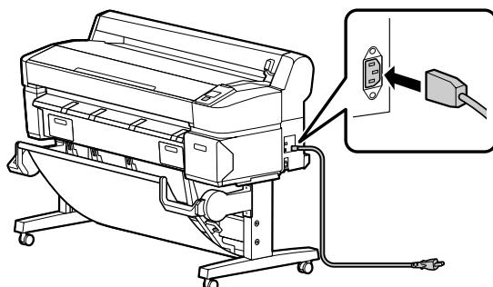
3. Plug the power cord into a properly grounded electrical outlet.
