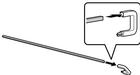
3. Slide the pole through the holes in the stabilizers and attach a plastic connector to the other end of the pole. Then, fasten the plastic connectors in place on each side of the stand.
