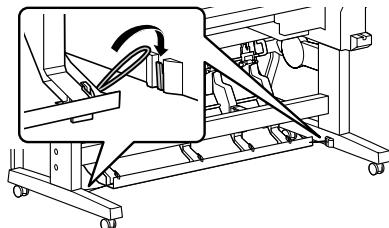
21. On the front side of the printer, slide the basket fabric all the way to the ends of the pole.
