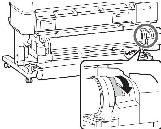
8. Push the secondary roll unit back into the printer.
