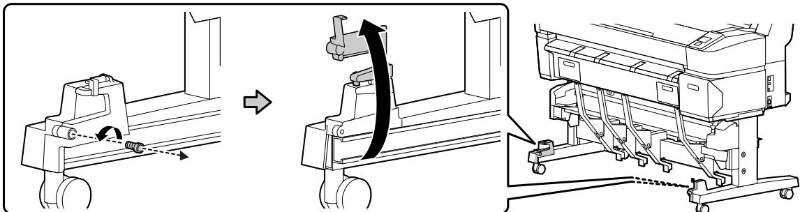
3. Insert the discs on the outside of the basket frame into the rails.
