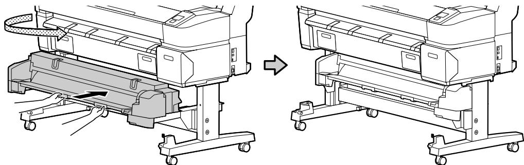
4. Insert the cable guide into the back of the second roll unit.
