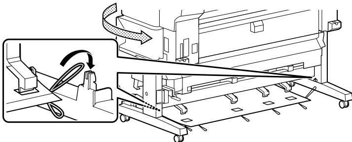
9. On the back side of the printer, pull the paper basket up so that the stack guides fit into the slots. Then, hook the loops around the pins on the back of the stack guides to hold the basket in place.
