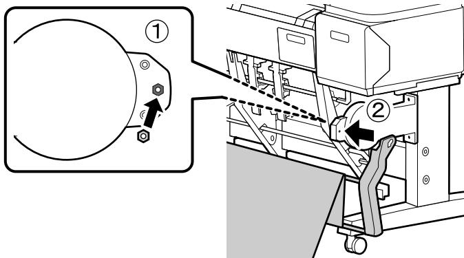
12. Insert the bolt sleeve through the basket arm and into the bolt hole. Insert the bolt into the bolt sleeve and tighten it. Repeat steps 11 and 12 on the left side of the printer.
