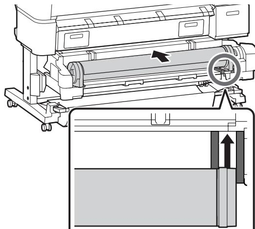
6. Insert the end of the roll paper into the paper slot and pull it through. Make sure the paper is free of slack and that the end is not folded. You hear a beep and the paper is automatically loaded.
