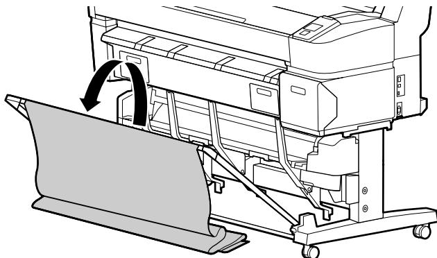
6. Open the clips on the basket, insert the loops and close the clips.
