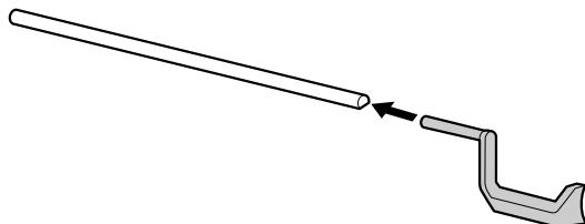
16. Insert the end of the round pole into the arm on the left side of the printer. Then, align the right basket arm with the mounting holes on the right basket holder.
