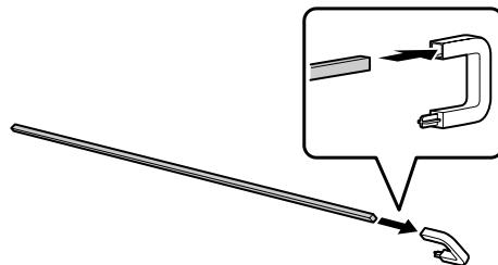
6. Slide the pole through the holes in the stack guides and attach a plastic connector to the other end of the pole. Then, fasten the plastic connectors in place on each side of the stand.
