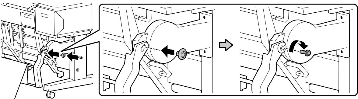
13. Attach the shorter arm to the inside of the basket holder on the left side of the printer. Use two nuts to hold the arm in place.
