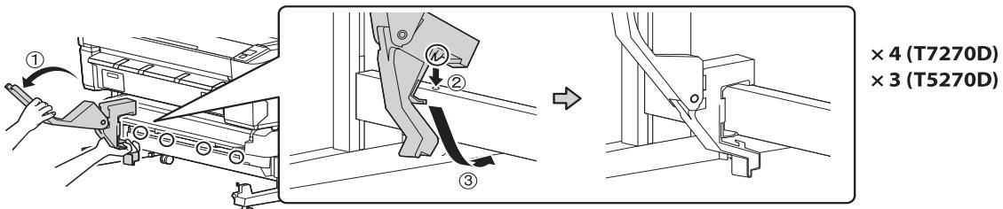
2. Remove the bolts from the front of the printer stand and then open the rail covers.
