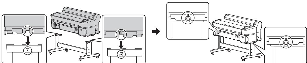
2. Attach the printer to the stand using three bolts.
