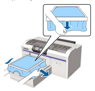
**Note:** The printer detects the highest part of the garment surface and adjusts the height accordingly. If there are any wrinkles, creases or slack near the inside edge of the frame, a platen height error
