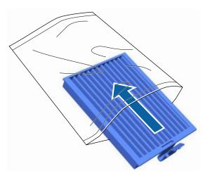
10. Install the new air filter into the printer as shown and press it down until you hear it click into place.
