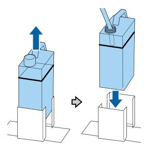
**Caution:** Verify that the waste ink tube is still inserted into the neck of the bottle. If the waste ink tube comes out of the bottle, waste ink will spill out.
