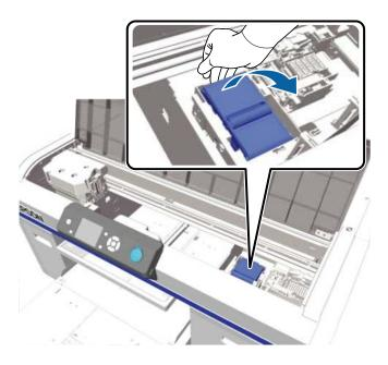
5. Grasp the wiper unit as shown and lift it out of the printer.
