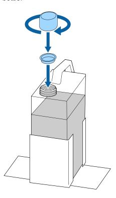
4. Remove the used waste ink bottle from the waste ink bottle holder and insert the new bottle. Make sure the new waste ink bottle is seated correctly in the waste ink holder.
