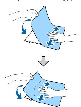
6. Peel off the grip pad backing from all the edges.
