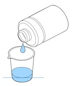
3. Place a cleaning swab or cleaning cloth in the ink cleaning solution and let it soak in. Make sure that the solution does not drip from the cleaning swab or cleaning cloth when you remove it from the cup.
