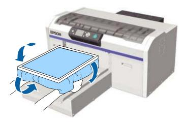
10. Reposition the platen frame a final time to make sure the garment is securely held down but not stretched.
