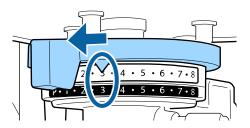
• When printing on T-shirts using the large garment, medium garment, small garment, or extra small garment platens with spacers a and b attached and a grip pad attached, select 4 on both spacers.
