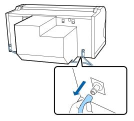
**Note:** Be careful when removing the waste ink tubes; waste ink may spill from the outlet or tube.
