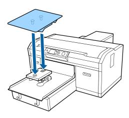
• If you are installing a medium grooved platen, make sure the cut out section faces the front as shown. Then go to step 3.
