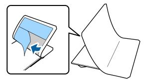
5. Carefully adhere the rest of the grip pad to the platen and rub each section to adhere it.
