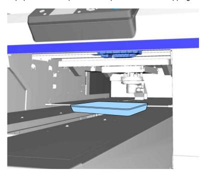
8. Look into the print head below the control panel. Wipe the edges at the front and rear of the nozzle surface with the cleaning swab as shown.
