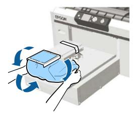
8. Reposition the platen frame a final time to make sure the garment is securely held down but not stretched.
