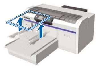
3. Load the T-shirt so that the shoulders are facing the front of the printer, as shown.
