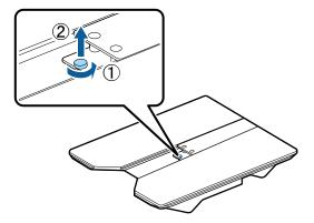
5. Slide the middle part of the platen back, then lift it up to remove it.
