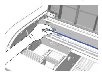
**Caution:** Do not touch the carriage shaft. Doing so may cause the printer to operate incorrectly.
