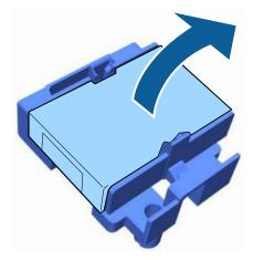
11. To remove the anti-drying cap from the printer, pull the lever toward you as shown here, and lift out the anti-drying cap.
