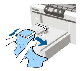
7. Tuck the sleeve around and under the frame so that it does not drape over the movable base.
