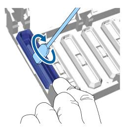
**Caution:** Make sure ink cleaner does not drip onto the anti-drying caps to the right of the suction cap. If any cleaner does drip, wipe it with a dry cleaning swab. If cleaner is left on the anti-drying caps, the print head nozzles could become clogged.
