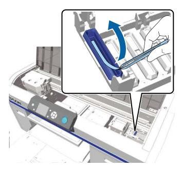
**Caution:** Use only the supplied plastic tweezers. Be careful not to damage the suction cap. If the suction cap is damaged, air may leak and the print head may become dry or difficult to clean.
