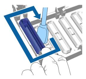
9. Wipe the top edge of the suction cap with a large cleaning swab dampened with ink cleaning solution.
