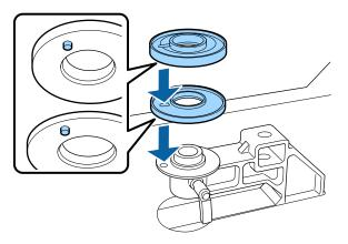
**Note:** Make sure the protruding sections of the spacers are aligned with the hole as shown.
