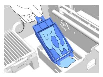
5. Place the used flushing pad into the bag that contained the new flushing pad.
