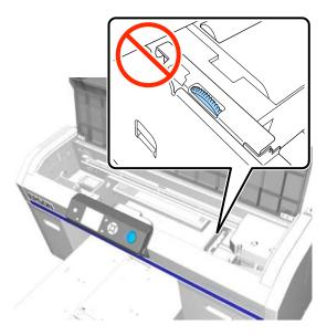
5. Wipe the metal border on the right of the flushing pad.
