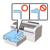
5. Tuck the T-shirt around the platen so that it does not drape over the movable base.
