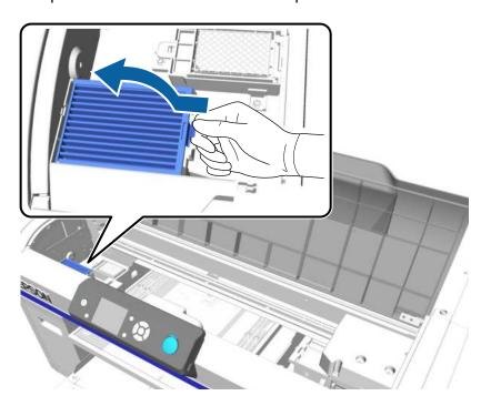
9. Place the used air filter into the bag you retained from the new air filter.
