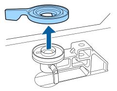
9. Remove or attach the spacers beneath the height adjustment lever.
