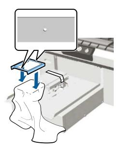
6. Gently pull the edges of the sleeve outside of the frame to remove any slack.
