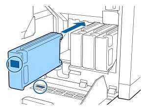
**Note:** Make sure that the color of the ink cartridge matches the color of the label on the printer.
