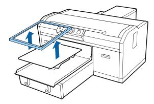
5. Place one sheet of A4- or letter-size plain paper on the center of the platen or grip pad. Secure the corners with tape.
