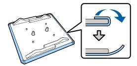
3. Flip the platen over and hold it down with one hand.
