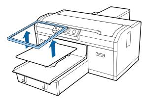
5. Place one sheet of A4- or letter-size plain paper on the center of the platen or grip pad. Secure the corners with tape.
