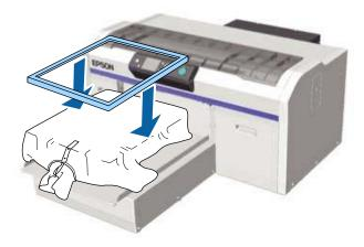
8. Gently pull the edges of the shirt outside of the frame to remove any slack.
