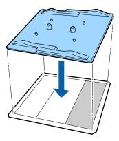
3. Flip the platen over and rub the section of the grip pad where you removed the backing to adhere it to the platen.
