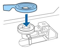
11. Reattach the parallel adjustment plate. Reinstall and tighten the screw that was removed in step 6 if you attached both spacers.
