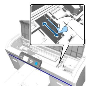
**Note:** Do not apply force to the gears shown below when cleaning. A malfunction may occur.
