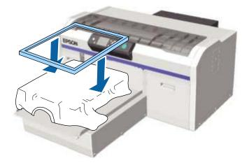
6. Gently pull the edges of the T-shirt outside of the frame to remove any slack.
