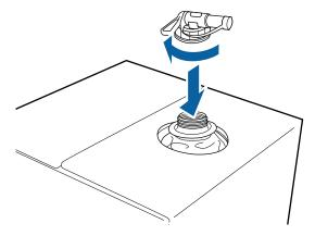
6. Remove the cap from the end of the tap and turn the lever until the hole is facing down.
