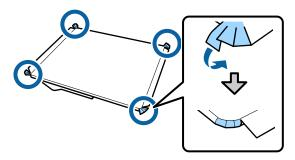
9. Fold over the short edges of the grip pad and adhere them to the back of the platen.
