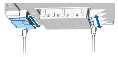
**Caution:** Do not touch the nozzle surface or the parts on the left side of the nozzles with the cleaning swab. A malfunction may occur.
