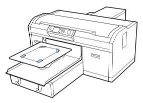
6. Set the height adjustment lever to the **P** position if you are using a platen or the **1** position if you are using a grip pad.
