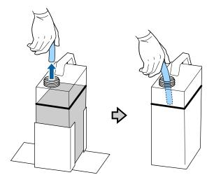
3. Place the inner and outer caps you removed from the new waste ink bottle on the used waste ink bottle.
