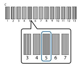
14. When **C** is displayed on the control panel, press the up or down arrow button to select the best pattern number, and press the **OK** button.
