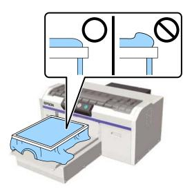
7. Tuck the T-shirt around the platen so that it does not drape over the movable base.
