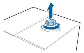
4. Remove the tap from the bag and turn the tap's handle section until the hole is visible as shown.
