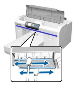
9. Wipe the parts on the left and right of the nozzle surface.
