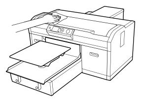
**Note:** To reduce ink mist buildup inside your printer, clean it regularly using a small amount of cleaning solution on a lint-free cloth. Gently clean the flat surfaces, print head cover, and inside the printer cover.
