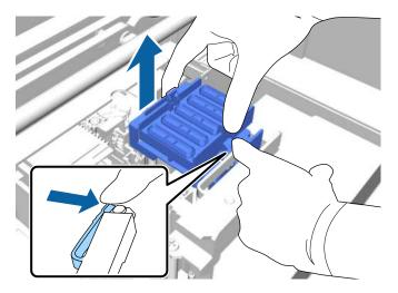
12. Place the cover on the old anti-drying cap and put it in the bag you retained from the new anti-drying cap.
