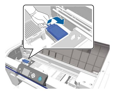
Caution: Lift the flushing pad carefully as ink could fly out if it is raised with too much force.
