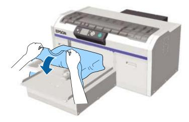
4. Gently pull the T-shirt over the edges of the platen to flatten it.
