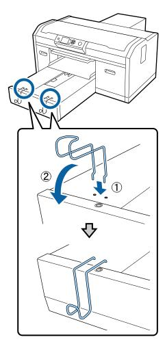
2. Make sure the front of the printer extends past the surface of the table or stand. Then hang the platen frame from the hooks.
