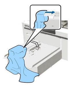
4. Gently pull the sleeve over the edges of the platen to flatten it.
