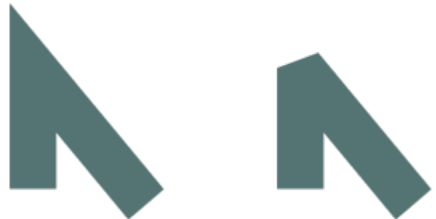
Lines meet at the same sharp angle. Left: The angle exceeds the miter limit, creating a pointed corner. Right: The angle is below the miter limit, creating a beveled corner.
