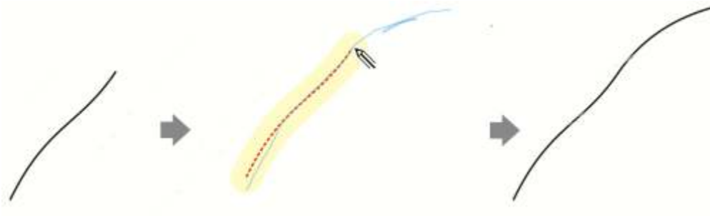
An existing stroke (left); A new stroke (in blue) is created close to the existing curve (middle); The existing stroke is extended and readjusted (right.)
