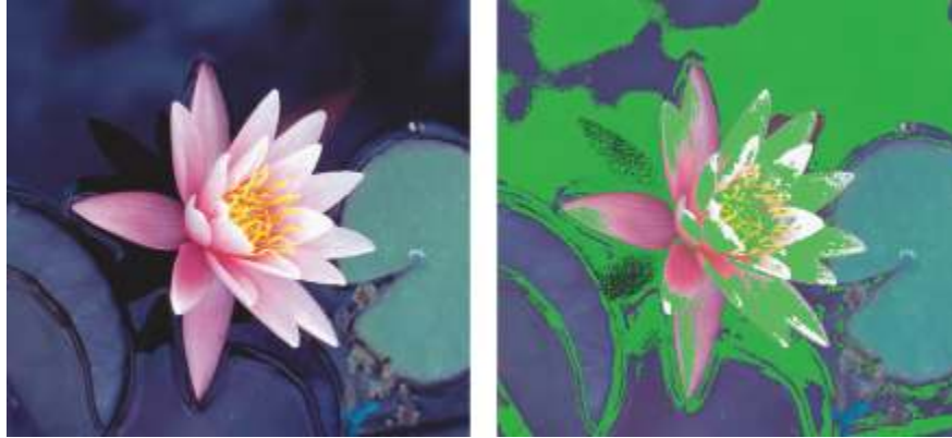
The gamut warning highlights colors that a printer or monitor cannot reproduce accurately.
