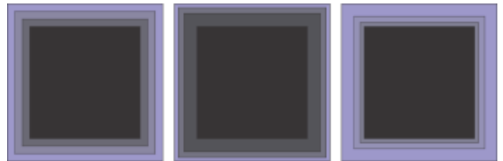
Left to right: Inside contour without acceleration, with lower acceleration, with higher acceleration
