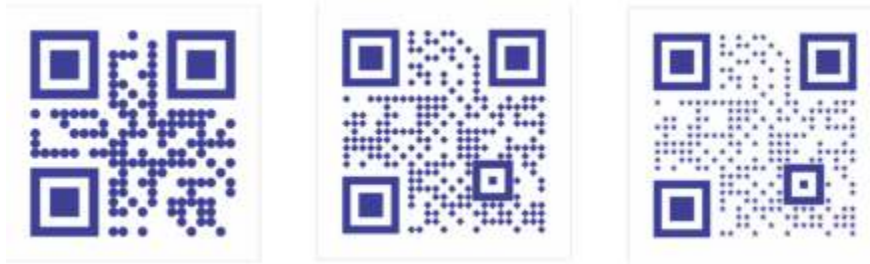
From left to right: QR codes with circular, diamond, and star pixel shapes
