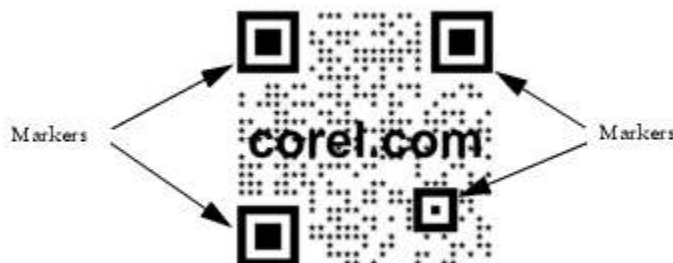
A QR code with customized pixel shapes and added text. The markers remain unchanged.
