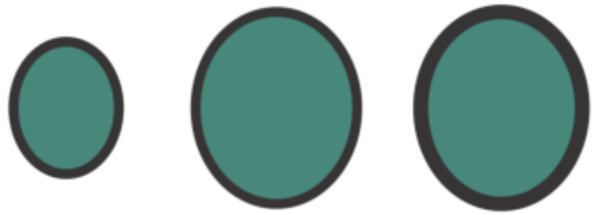
Left to right: Original object; scaled object with Scale with object disabled — there is no change in the outline thickness; scaled object with Scale with object enabled.
