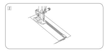
Attach the zipper foot with the pin on the right. Sew through all the layers from the end of the zipper opening, guiding the zipper teeth along the edge of the foot 3 Stop the machine 2" (5 cm) before the foot reaches the slider on the zipper tape. Lower the needle into the fabric, and raise the foot.
