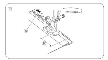
Open the zipper, then lower the foot and stitch the remainder of the seam.
