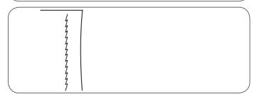
This stitch is a narrow stretch stitch designed to eliminate puckering on knit fabrics and bias seams, while permitting the seam to be pressed completely open flat.
