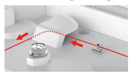
> Place the end of the thread down along the duct.
