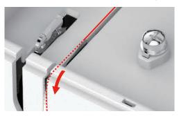
> Guide the thread downwards around the thread take-up lever cover.
