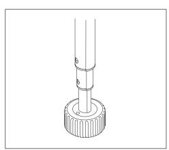
Monopod or Bi-Pod, check to make sure your legs are fully locked and secure. Apply downward pressure to the top of your unit to confirm your legs are at their full strength. If there is any leg slide, the Rubber Non-Slip Foot or Foam Rubber Collar for Final Height Adjustment must be tightened further in a clockwise direction to fully lock in place.
