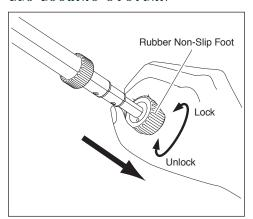
To release the legs, grasp the Foam Rubber Comfort Grip in one hand and the Rubber Non-Slip Foot in the other hand. TWIST the Rubber Non-Slip Foot in a counter-clockwise direction to unlock.
