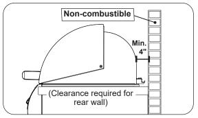
Fig. 18-1 Clearance 'A' Diagram
