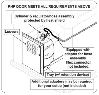
Fig. 14-3 Optional door w/ tank tray & louvers
