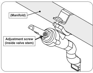
Fig. 52-1 Valve adjustment screw location
