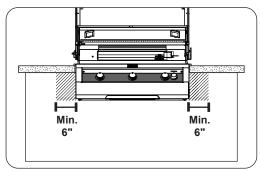
Fig. 19-1 Control panel clearances
