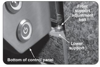
Fig. 29-1 Front support adjustment bolts
