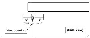
Fig. 12-2 Vent openings clearance
