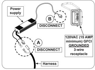
Fig. 48-1 Perform system reset
