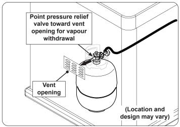
Fig. 7-2 Vapour withdrawal detail
