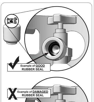
Fig. 9-1 Inspect rubber seal
