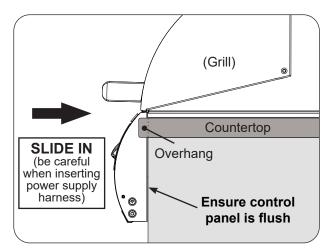
**Fig. 28-3** Slide in unit (ensure flush)
