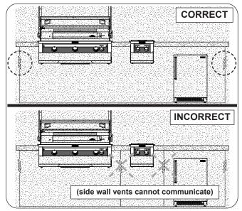
Fig. 12-1 Correct / Incorrect side wall venting
