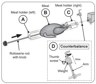
Fig. 42-3 Assemble rotisserie rod for cooking
