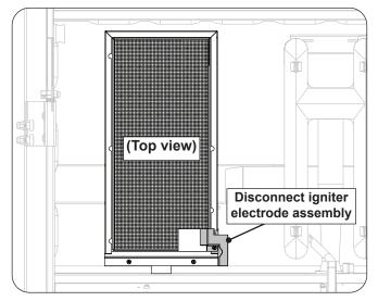
Fig. 48-4 Infrared burner removal
