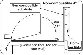
Fig. 18-2 Clearance 'B' Diagram
