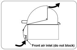
Fig. 19-2 Airflow diagram
