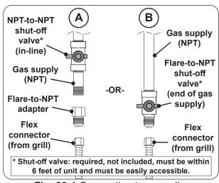
Fig. 30-1 Connecting to a gas line
