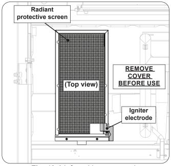
Fig. 43-1 Infrared burner overview
