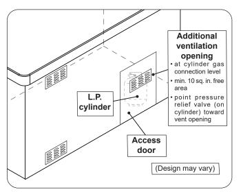
Fig. 14-2 Additional vent opening for L.P. cylinder
