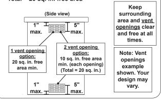
Fig. 12-3 Natural gas ventilation detail
