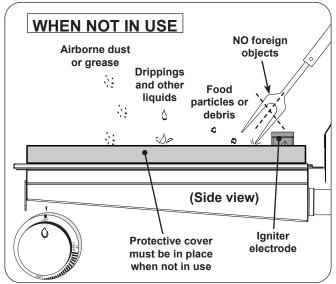
Fig. 43-2 Infrared burner - WHEN NOT IN USE
