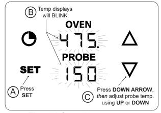
Fig. 40-2 Set probe temperature
