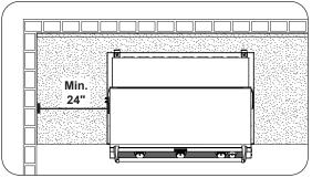
Fig. 18-5 Side/corner wall clearance
