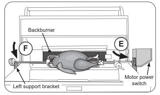
Fig. 42-4 Attach Rotisserie rod to motor
