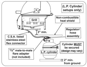
Fig. 14-1 L.P cylinder orientation (if applicable)
