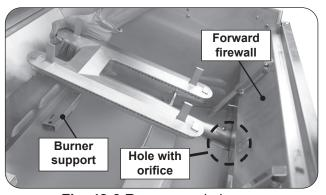
Fig. 48-3 Remove main burner
