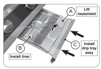
Fig. 32-3 Install drip tray
