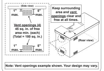
Fig. 13-2 Remote LP ventilation detail
