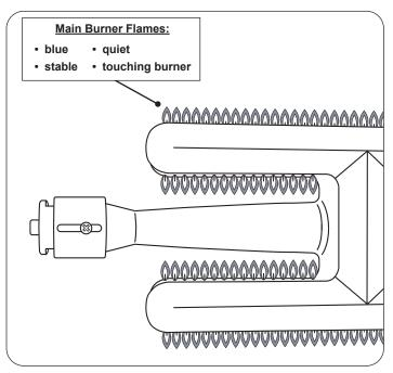
Fig. 51-1 Proper flame appearance
