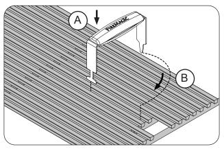
Fig. 32-1 Install cooking grids
