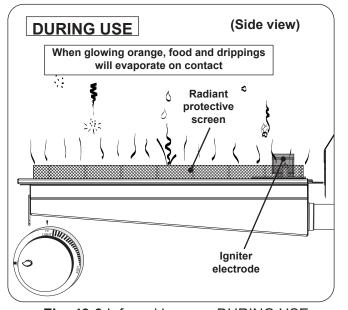
Fig. 43-3 Infrared burner - DURING USE
