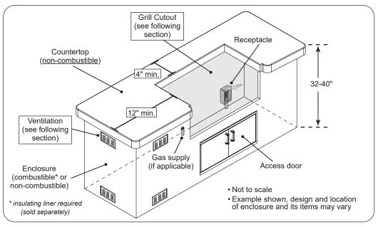
Fig. 11-1 Enclosure specifications
