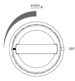
**Warning**: Before Lighting, please make sure that the control knob is in the off position and the regulator assembly is in good condition.
