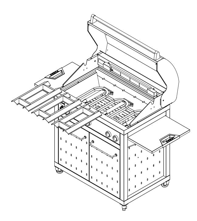
Install the cooking grates into the the firebox\*. The large grates should be installed with the flat edge towards the outside of the grill.
