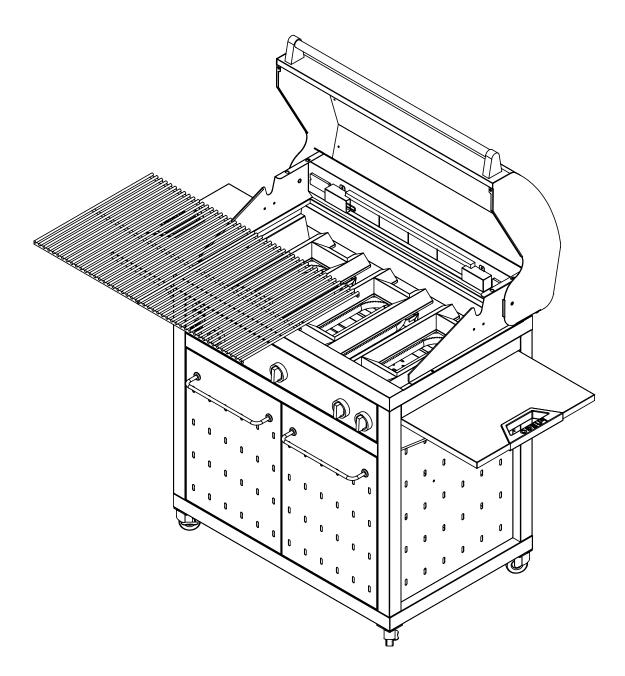
Install the warming rack into the firebox by installing the rear legs first then rotating forward to set the front legs into place.
