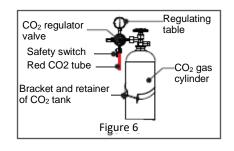
c) Using the wrench, tighten the CO<sub>2</sub> regulator table valve with the hex nut port to the gas outlet of the CO<sub>2</sub> tank (See Figure 6).
