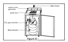
so that the raised bottom edge contacts the edge of the cabinet. Finally, lift the keg handle to raise the keg to the level of the floor of the cabinet and push the keg into place.
