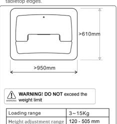
Ensure that the surface that you place the desk riser on is strong enough to support the desk riser and any equipment you are planning on using.
