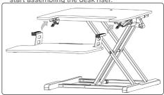
Lock the keyboard tray into place using the latches.
