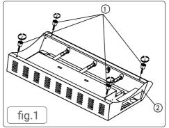
Attach the feet to the burner unit (fig.1).
