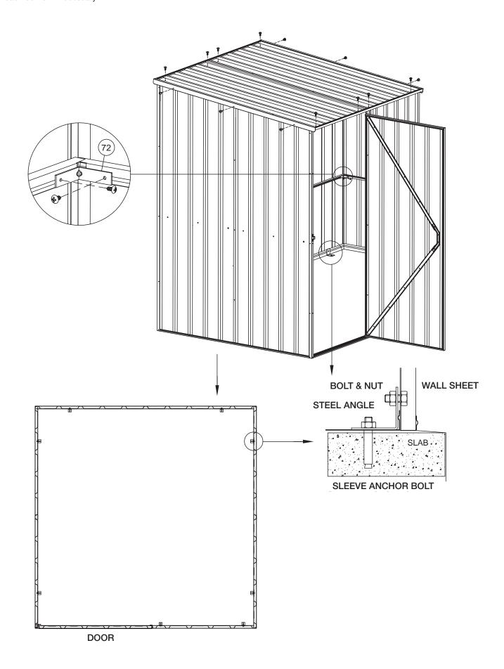
Apply channel safety cover (L type) to part 31 (channel) and channel safety cover (R type) to part 33R (channel). Also apply the self-tapper covers to screw ends visible in the walls on the inside of the shed as per the diagram below.
