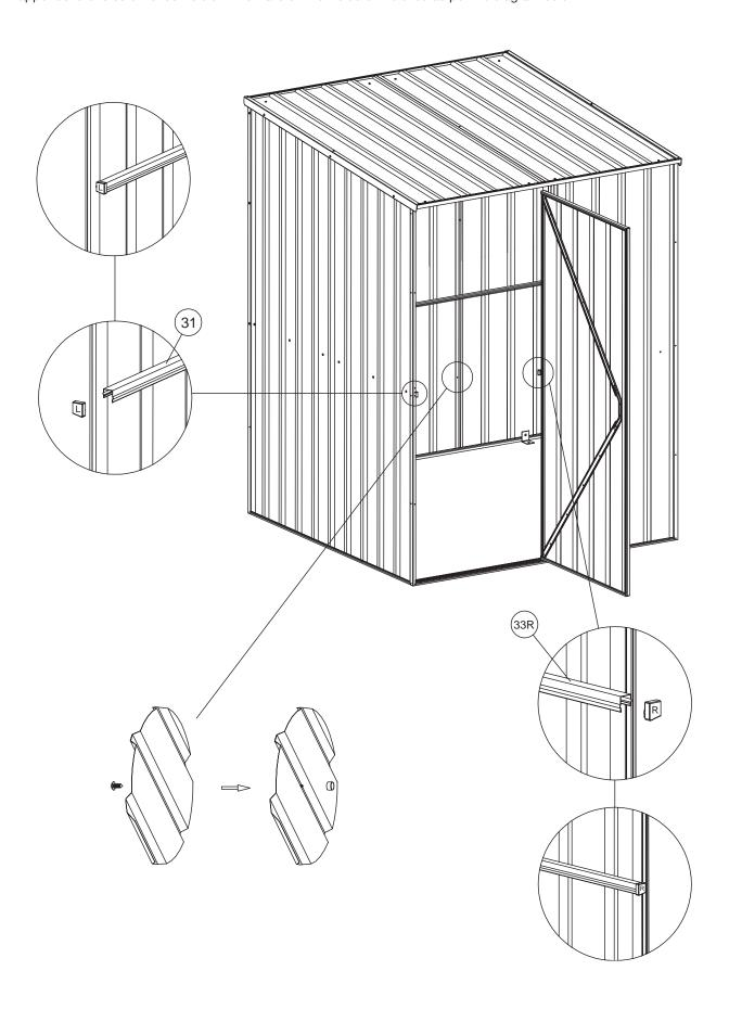
The door can be hinged on the opposite side as well. Align the door with the edge and make holes using a cordless drill. Remove the pins from the hinges and reverse their direction before you attach the door. If you are concerned about the visibility of any predrilled holes, you can fill them with rivets. Perform the same procedure for the pad bolt.
