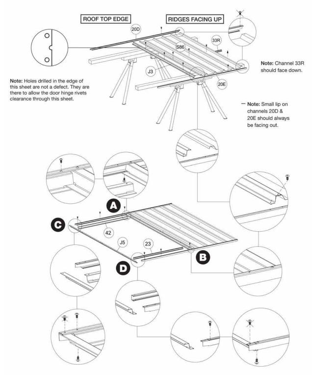
Fit part J5 (jamb), part 42 (jamb) and part 23 (bottom channel) and fix them with the self tapping screws (except those marked with a cross). Make sure both joins (diagrams A and B) are fixed the same followed by diagrams C and D.
