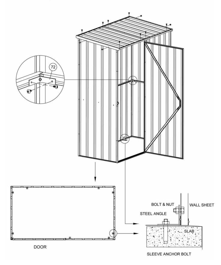
For safety apply channel safety cover (L type) to part 32 (channel) and channel safety cover (R type) to 33R (channel). Also apply the self-tapper covers to screw ends visible in the walls on the inside of the shed as per the diagram below.
