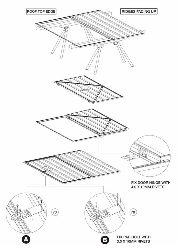
Attach the two side walls to the back wall, then fix the front wall followed by the roof. Fix all of these components together using the provided self-tapping screws. Fix the pad bolt keeper with the provided 16mm self-tapping screws (diagram A) or using rivets (diagram B) at this stage as well. Also attach parts Z37, Z38, Z39 and Z40 (corner brace) to each corner using the self-tapping screws (diagram A) or using rivets (diagram B) provided.
