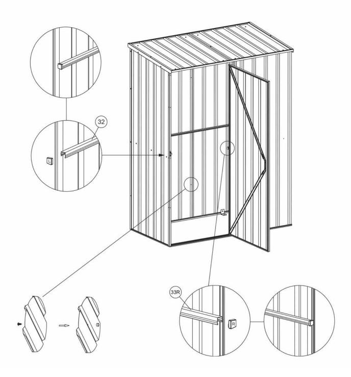
The door can be hinged on the opposite side as well. Align the door with the edge and make the holes using a cordless drill. Remove the pins from the hinges and reverse their direction before you attach the door. If you are concerned about the visibility of any pre-drilled holes, you can fill them with rivets. Perform the same procedure for the pad bolt.
