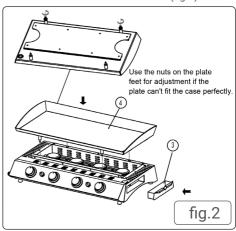
• Attach the plancha to the burner unit (fig.2.4). Insert the drip tray (fig.2.3).
