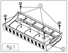
· Attach the feet to the burner unit (fig.1).
