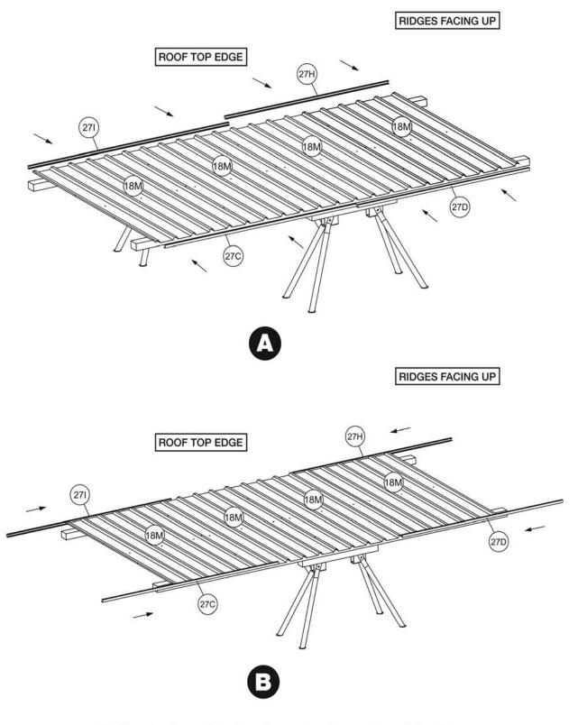
Tip: If panel and screw holes do not line up, try pulling panel to match up holes.
