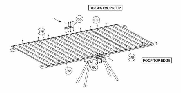
Enhance the structural strength by applying part 66 (channel connectors). Note that screws are applied to both sides of the connectors as per Step 3.
