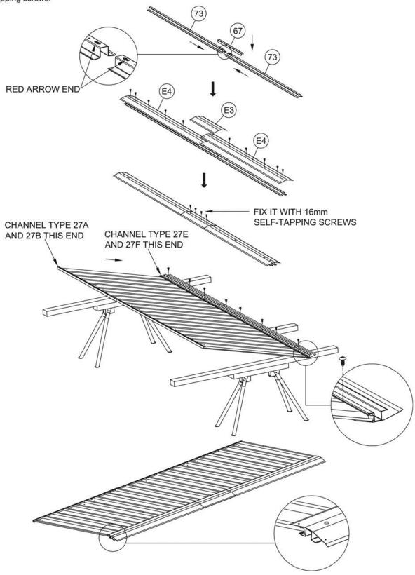
Slide the side of the roof panel with channels 27E and 27F into the ridge beam.
