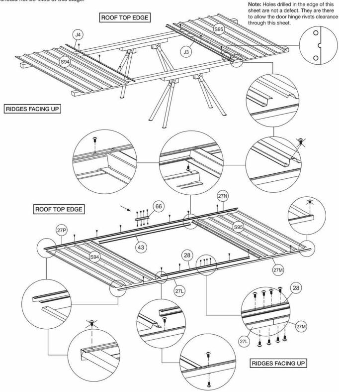
Fix parts 27P and 27N (top channels), part 43 (jamb), and parts 27L, 27M, and 28 (bottom channels) using self-tapping screws. Enhance the top channels by applying part 66 (channel connector) and fix screws through both sides. Please note: for parts 27P, 27N, 27L and 27M the small lip should be facing out to stop water building up and leaking into shed.
