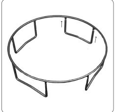
• Lift the frame and insert assembled legs into the T sockets from the underside of the ring frame. (The legs will be bolted on when the safety net legs are added).
