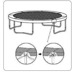
• Rotate the padding so the tie straps line up with the leg positions. Tie the padding around the frame and leg, this will help to stop the padding from moving.
