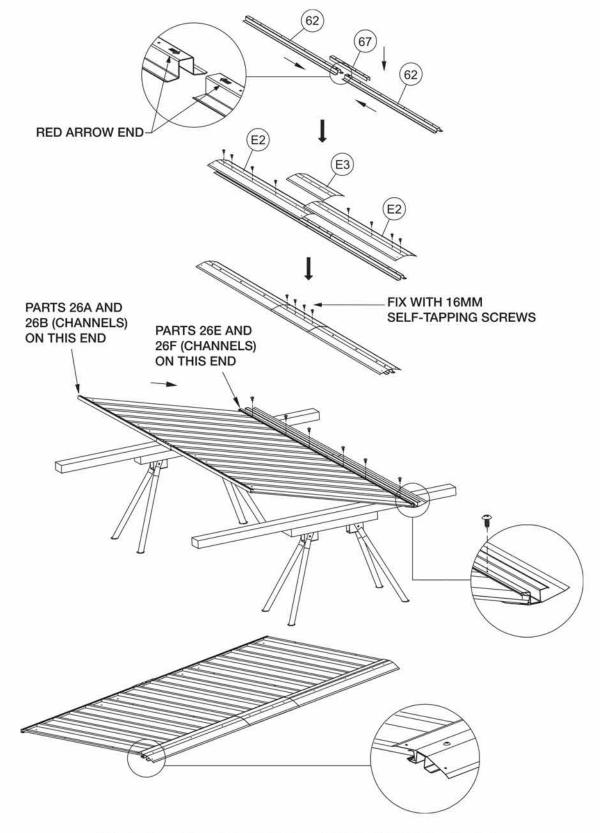
Slide the side of the roof panel with channels 26E and 26F into the ridge beam.
