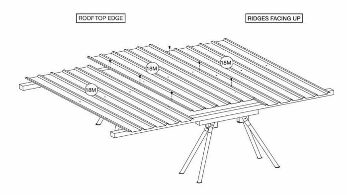
Tip: If panel and screw holes do not line up, try pulling panel to match up holes.
