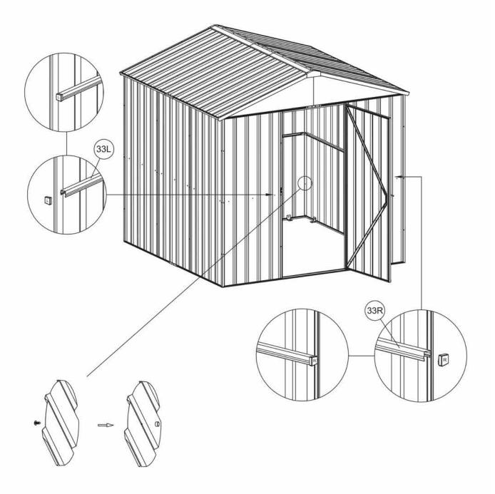
The door can be hinged on the opposite side as well. Align the door with the edge and make holes using a cordless drill. Remove pins from the hinge and reverse their direction before you attach the door. If you are concerned about the visibility of any pre-drilled holes you can fill them with rivets. Perform the same procedure for the pad bolt.
