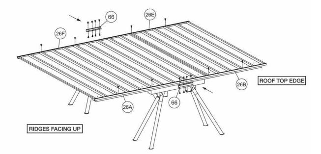
Enhance the structural strength by applying part 66 (channel connector). Note that screws are applied to both sides of the connectors.
