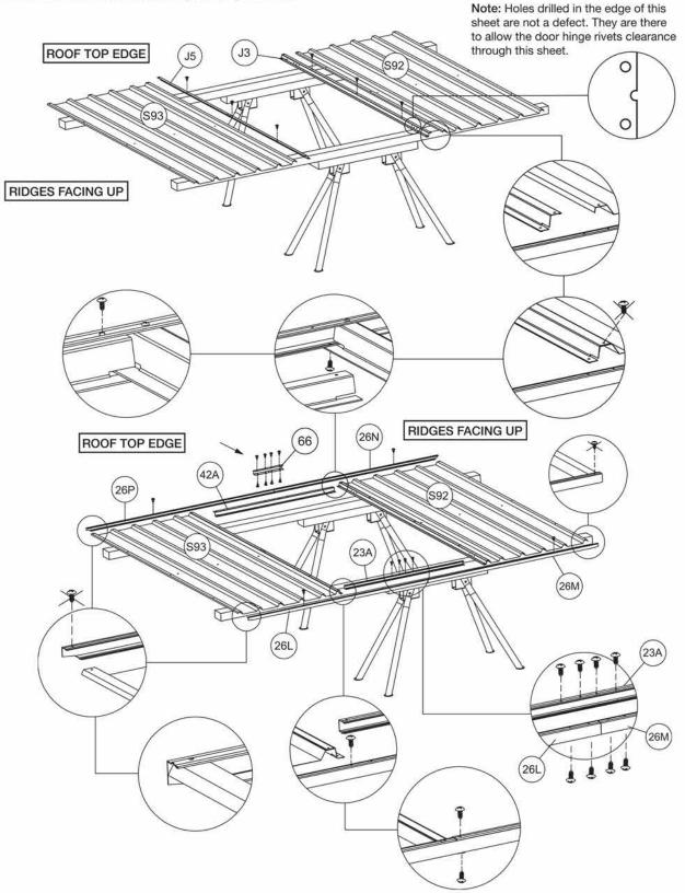
Fix parts 26P, 26N (top channels), 42A (jamb), 26L, 26M, and 23A (bottom channels) with self-tapping screws. Enhance the top channels by applying part 66 (channel connector).
