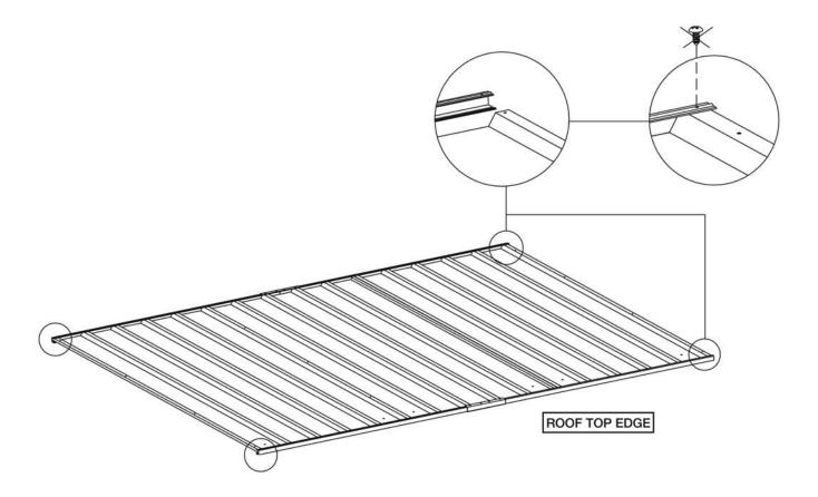
Fix parts J3 and J5 (jamb) to parts S92 and S93 (sheeting) with self-tapping screws as per diagram below. **NOTE:** All screws marked with a cross should not be fixed at this stage. Make sure the small lip on the channel is always facing out. This ensures rain water cannot build up inside your shed.
