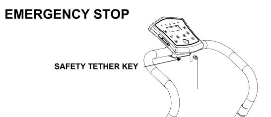
Before beginning a workout session ensure that the Safety Tether Key is properly placed onto the Computer Console and the Safety Clip is securely attached to an article of your clothing. If you fall the clip will pull out the **SAFETY TETHER KEY** from the Computer Console and the running belt will stop immediately for emergency stop, helping to prevent injury.
