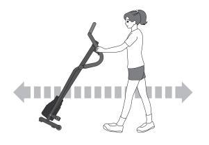
The unit can be carefully tilted onto its transport wheels for easy moving and storage. With the treadmill in the folded locked position, firmly grasp the Handlebar with both hands. Next, carefully tilt the treadmill back until it rolls freely on the Transport Wheels.
