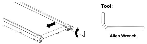
If the running belt is slipping during use, turn off and unplug the treadmill. Using the Allen Wrench provided, turn both left and right rear roller adjustment bolts 1/4 turn clockwise, then turn the main power switch back on and run the treadmill at a speed of 8-10 KPH. Run on to the running belt to determine if the belt is still slipping. Repeat this procedure until the belt no longer slips.
