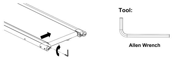
If the running belt is shifting to the right, then turn the right adjustment bolt 1/4 turn clockwise, and the belt should start to correct itself. Keep turning the adjustment bolts until the running belt is properly centered.
