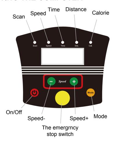
1.Plug in the power, put the Emergency Stop Switch on the position of Control Panel, open the switch, digital lamp and LED full-light, the control panel will beep to indicate the Panel is on and enter into Standby Model, the digital display "-.-.-." Press the On/Off button, the Treadmill will start work in Manual Mode, press On/Off button again, The Treadmill re-enter standby mode.
