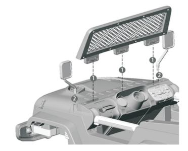
1. Put the wind shield into the frame and fixed it
