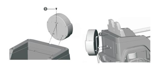
1. Install the Storage box, and fix it with  $Ø4 \times 10$  screw
