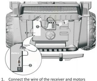
2. Open the cushion and insert wires into the socket **Red to red , black to black**
