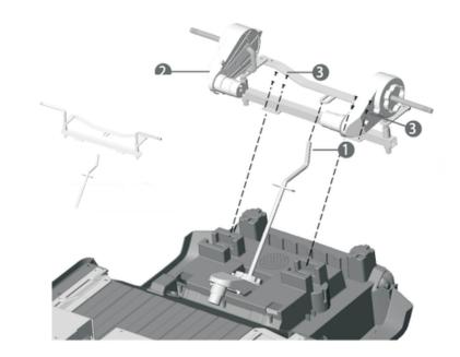
Insert the steering rod into the hole of the steering frame.
