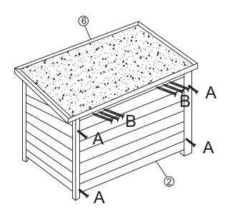
Secure back panel part② with 4x bolt&nut (A). Attach roof part⑥, secure by using 6x screw(B) at back.
