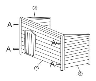
Connect part①, part③ and part④ together, secure by using 4x bolt&nut (A).
