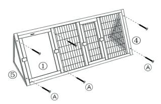
Secure left panel part<sup>(5)</sup>,middle panel part<sup>(3)</sup> and right panel part<sup>(4)</sup> by each using 2x screw(A), total 6x screw (A).
