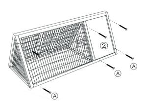
Secure back panel part<sup>(2)</sup> by using 6x screw (A).
