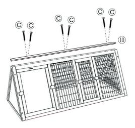
Attach part<sup>1</sup> to the top, secure with 6x screw(C).
