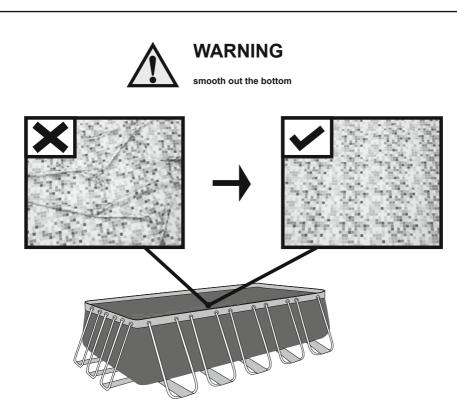
Put 1" to 2" water in the pool to cover the floor. Once pool floor is slightly covered, gently smooth out all wrinkles. Start in the center of the pool and work your way clockwise to the outside.
