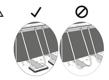
Do not assemble on soft lawn. If you must assemble the pool on a soft surface, timber boards must be placed under the feet of the vertical supports to spread the load.
