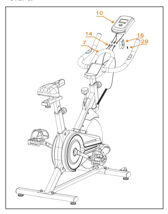
FIX THE PLASTIC MONITOR POST (16) TO THE HANDLEBAR (7) WITH SCREWS (29). PUT THE MONITOR (10) TO THE POST (16), THEN JOINT THE SENSOR WIRE.THEN JOINT THE SENSOR WIRE (14). THE INTERFACES ARE MATCHING.
