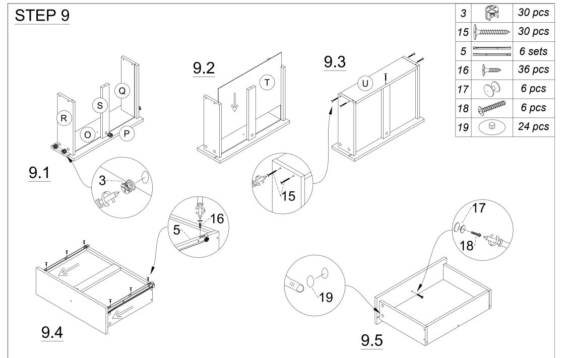
PLEASE PUSH THE DRAWER SLIDES UNTIL THE END ACCORDING TO THE ARROW'S DIRECTION SHOWN ABOVE.
