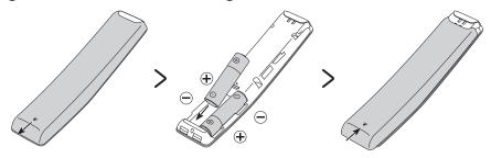
To install the batteries, push the rear cover open in the direction of the arrow at the bottom of the illustration, and then insert the batteries as shown in the figure. Make sure that the positive and negative ends are facing in the correct direction. Close the rear cover as shown.
