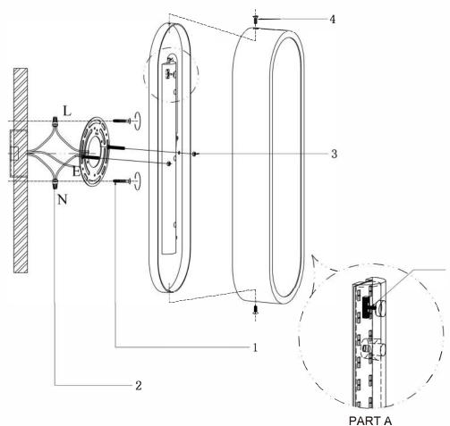
Ensure the power has been cut-off then open the fixture, use the switch on the LED board to adjust it to the CCT you want,"W" is 3000K,"M" is 4000K,"C" is 5000K
