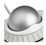
Optical tracking technology delivers precise cursor movement for superior accuracy, so you can get where you want on the screen quickly with less hand movement, improving productivity and efficiency.
