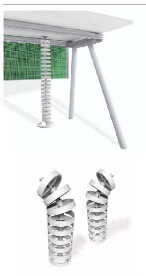
CMS Cirqlate is specifically designed for cable protection when bringing power and data cables from the floor or ceiling to the work surface. It comprises three separate compartments for cable distribution. Because all components clip together simply, on-site adjustment is easy and quick by the addition or removal of extra pieces.
