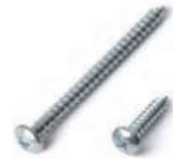
Fastening screws High quality wood screws are sufficient for fixing the grates to a timber joist structure. However with the Ryno aluminium substructure, stainless steel screws should be used to ensure no corrosion occurs.
