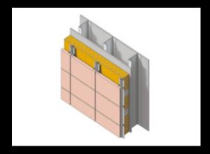
In line with the Building Control Alliance Technical note 18; 'use of Combustible Cladding Materials on residential buildings paragraph 12.7 of AD B2' - use materials of limited combustibility throughout the cladding system.
